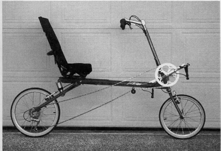
Mark Colliton's RCN R32 test bike #2 with no front suspension. Note: Bottom bracket is one inch lower than the suspension bike
